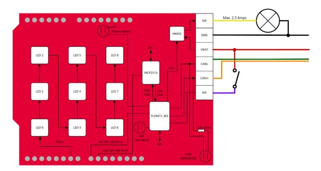
All CAN communication is done on 500 kBaud/s bus speed. After start-up, following features can be used:
