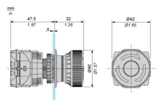
(e) Clamping thickness: 1 mm to 6 mm / 0.03 in to 0.24 in
