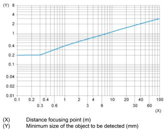
Minimum size of the object to be detected (mm)
