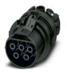
Circular connectors (cable-side), Contact insert, type: Release with tool or by hand (see accessories), housing material: PPE, color: black, number of positions: 5, min. conductor cross section: 1.5 mm<sup>2</sup>, max. conductor cross section: 6 mm<sup>2</sup>, nom. voltage: 690 V AC, rated current: 35 A, Connection method: Screw connection, Type of contact: Socket
