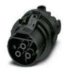
Circular connectors (cable-side), Contact insert, type: Release with tool or by hand (see accessories), housing material: PPE, color: black, number of positions: 3, min. conductor cross section: 1.5 mm<sup>2</sup>, max. conductor cross section: 6 mm<sup>2</sup>, nom. voltage: 690 V AC, rated current: 35 A, Connection method: Screw connection, Type of contact: Socket
