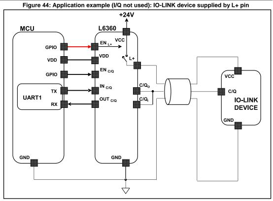
In case of very high capacitive loads on L+ the IC could trigger the thermal protection threshold. The table below shows the maximum capacitance that L+ can supply without triggering the thermal protection.
