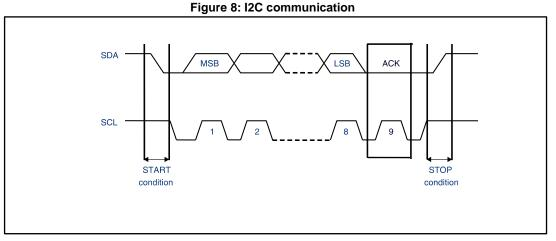
Each byte is followed by an acknowledgment bit as indicated by the A or A blocks in the sequence. A START condition immediately followed by a STOP condition (void message) is a prohibited format.
