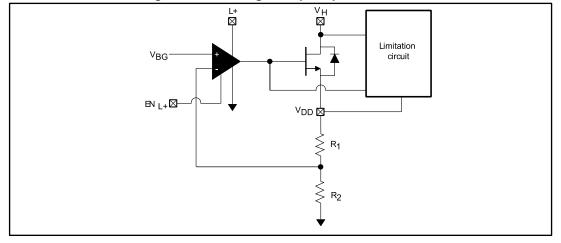
Figure 42: Linear regulator principle schematic
