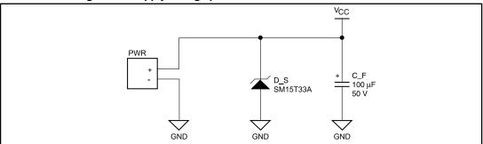
Performance of the above mentioned example is limited and does not include reverse polarity protection. It is just a cost-effective solution.
