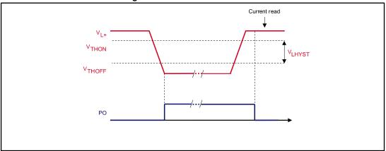
Figure 10: Power-on bit behavior
