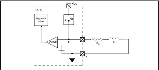
When a high-side driver turns off an inductance, a reversed polarity voltage appears across the load. The output pin (L+) of the power switch becomes more negative than the ground until it reaches the demagnetization voltage,  $V_{demag}$ . The conduction state of the power switch Q1 is linearly modulated by an internal circuitry in order to keep the voltage at C/Q
