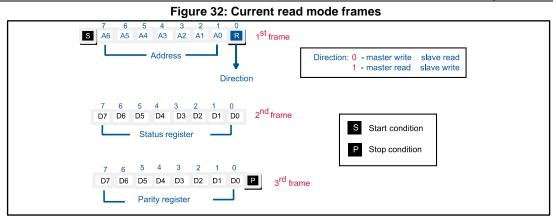
When a "read request" comes from the microcontroller (it is configured as master receiver), the IC (slave transmitter) sends the contents of the status and parity registers.
