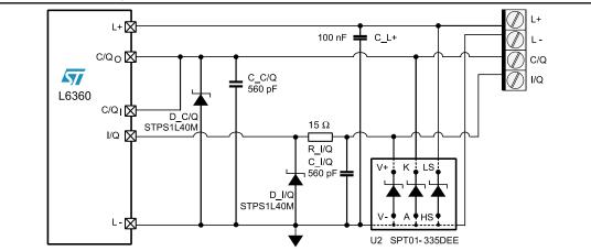
Table 36: IO-Link and SIO application extended protection component description
