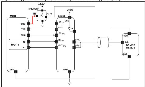
Figure 45: Application example (I/Q not used): IO-Link device supplied by single channel IPS
