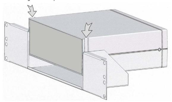
4. Fully screw the 2 M4 x 10mm screws (supplied) into the threaded bosses, keeping gentle pressure on the front corners of the case as the screw threads into the case push-rivet hole.
