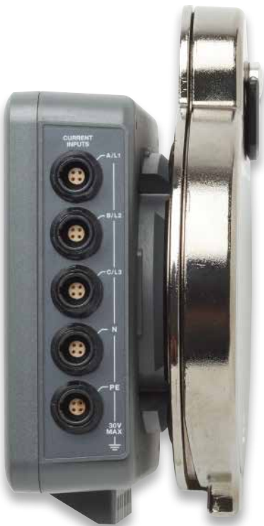
Current inputs for installing measurement probes inside the electrical panel
