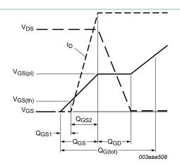
Fig. 15. Gate charge waveform definitions
