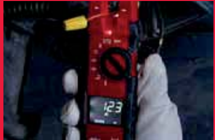
Built-in Voltage Detector
