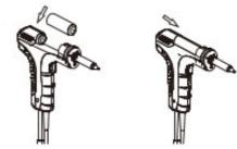
• The suction nozzle/tip can be removed for cleaning by unscrewing the knurled nut and sliding off the barrel. The nozzle/tip can then be pressed out of the barrel.
