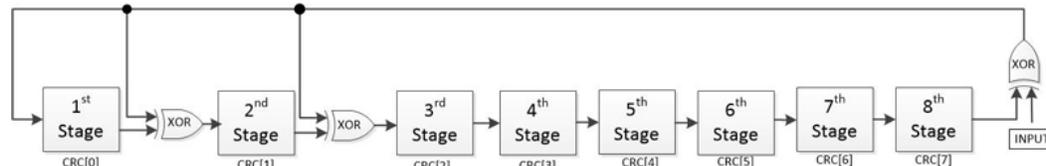
Figure 6. PEC generator for  $CRC = X^8 + X^2 + X^1 + 1$ .
