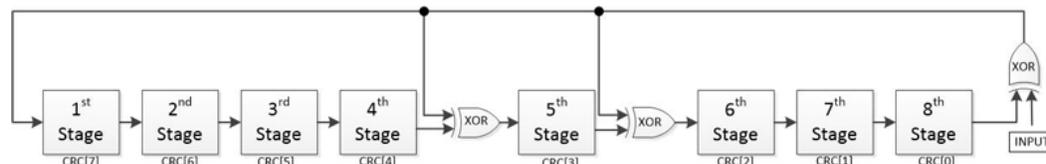
Figure 5. CRC generator for  $CRC = X^8 + X^5 + X^4 + 1$ .
