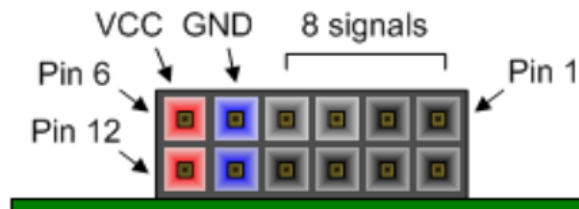
Figure 8 – UART/BLE Female Connector (viewed from board edge)
