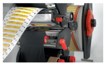
Time-saving and intelligent: double-sided printing with different content in one work step.
