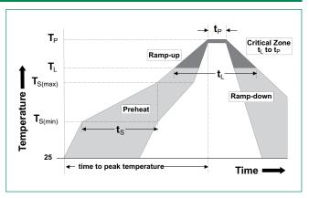
All temperature refer to topside of the package, measured on the package body surface
