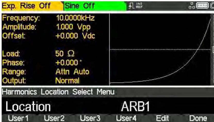
The instrument is capable of creating waveforms by the addition of sine wave harmonics. Up to 16 harmonics can be used, chosen from up to the 50<sup>th</sup> order. The amplitude and phase can be individually set for each harmonic. Harmonic waveforms can also be created or edited in the Waveform Manager Plus V4.13 Windows application supplied on the website: [www.aimtti.com](http://www.aimtti.com)
