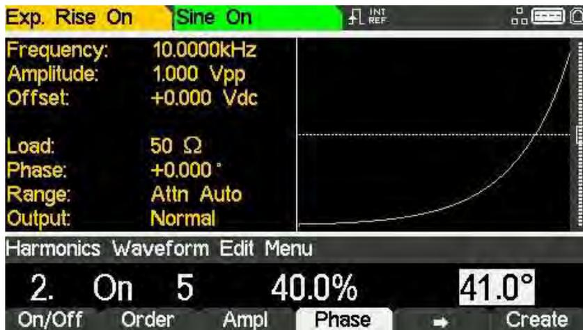
To output the harmonic waveform, select ARB as the carrier waveform and then select the user-defined arbitrary waveform where the harmonic is stored as the output from the **Arbs** menu under **Load**.
