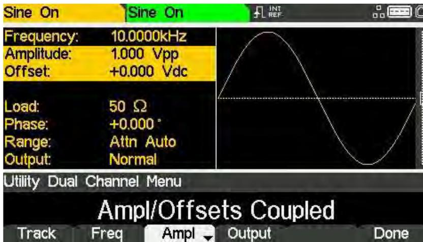
To enable or disable output coupling press the **Output** soft-key.
