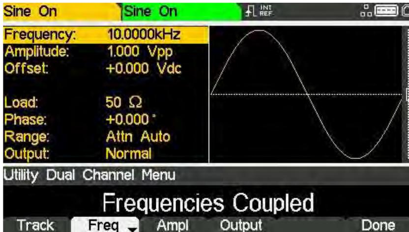
When entering frequency coupling modes, the instrument will automatically phase align the channels. The phases may become misaligned by subsequent parameter changes. To realign the phase at any time, press the **Align** soft-key from the carrier- output menu.
