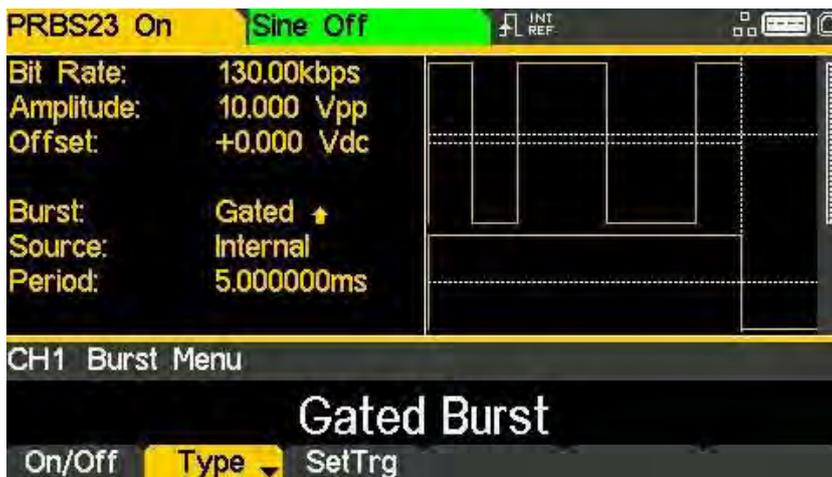
The currently selected type will appear in the Edit Box, the **Burst** field in the Parameters Box will show the type and the Graph Box will show the trigger waveform below a representation of the carrier waveform with the burst type applied.
