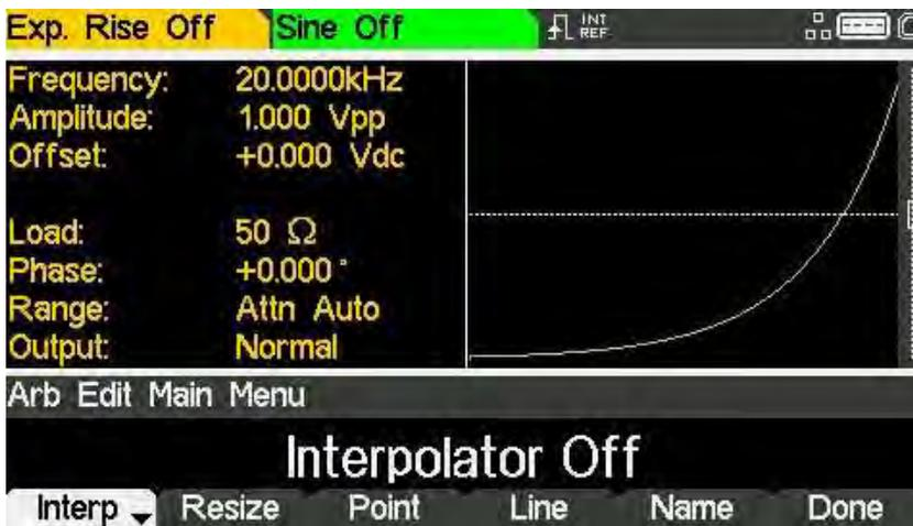
With **Interpolator On** selected linear interpolation will be used as points are added, this is most appropriate for waveforms which are more sinusoidal in nature.
