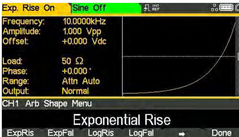
The soft-keys allow access to all of the arbitrary waveforms in the instrument.
