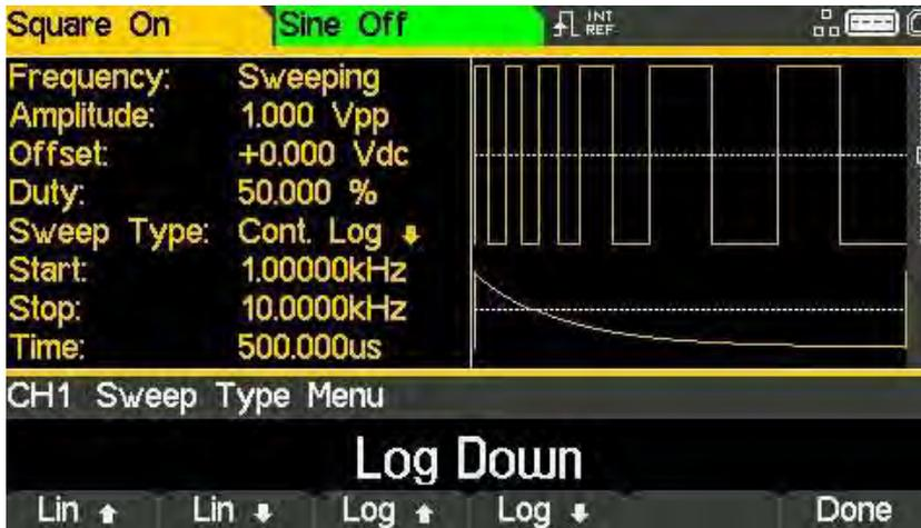
The arrows indicate up or down sweeps. With any of the **Lin** types selected the sweep changes the frequency at a linear rate; with **log** types selected the sweep spends an equal time in each frequency decade. The up arrows indicate a sweep from start frequency to stop frequency. The down arrows indicate a sweep from stop frequency to start frequency.
