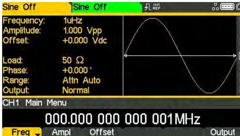
With the edit cursor positioned at the required digit the knob may be rotated left or right to decrement or increment the digit. As the value passes between 9 and 0 the digits to the left will also change. In this way it is possible to set any legal value for the parameter.
