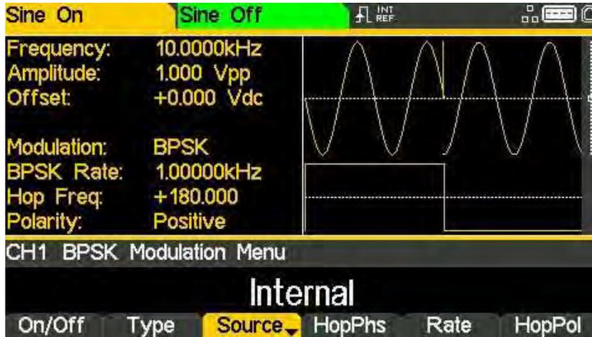
External will use the signal present at the TRIG / COUNT (DC) IN connector and the Rate parameter will no longer be editable. The Graph Box will show a switching carrier and a square-wave as the modulating waveform irrespective of the source of the switching signal.
