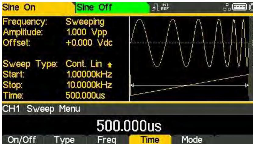
The Parameters Box now shows the current sweep parameters of **Sweep time**, **Start**, **Stop** and **Time**, and **Sweeping** is shown in the **Frequency** field. The Graph Box shows the sweep waveform type below a representation of the swept carrier waveform. The Edit Box contains the selected parameter, in this case sweep time.
