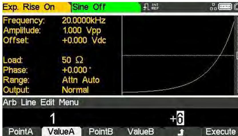
The **PointB** and **ValueB** soft-keys are used to set the second point. The line is drawn in the actual waveform by pressing the **Execute** soft-key after which the instrument will return to the top-level edit menu.
