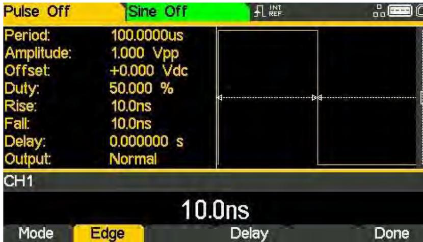
The edge time represents the time between the 10% and 90% points on the pulse edges. Rise time and fall time can be coupled or adjusted independently.
