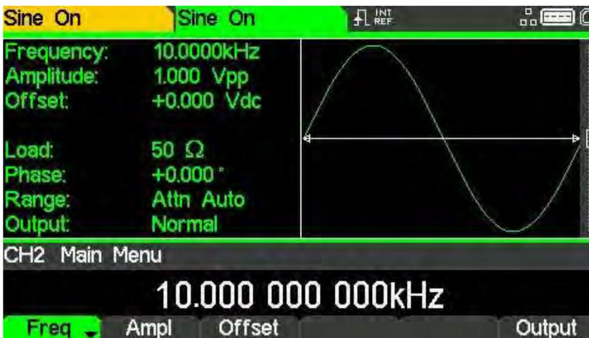
Any channel specific set parameters will always be shown in the specified colour for that channel.
