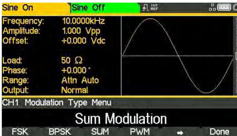
Press On/Off soft-key to apply the selected modulation.
