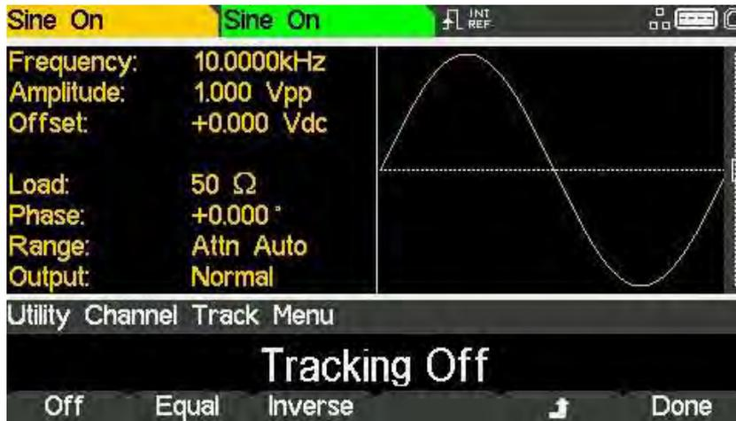
With Tracking Off the two channels behave independently and changes to parameters on one channel do not affect the other channel.
