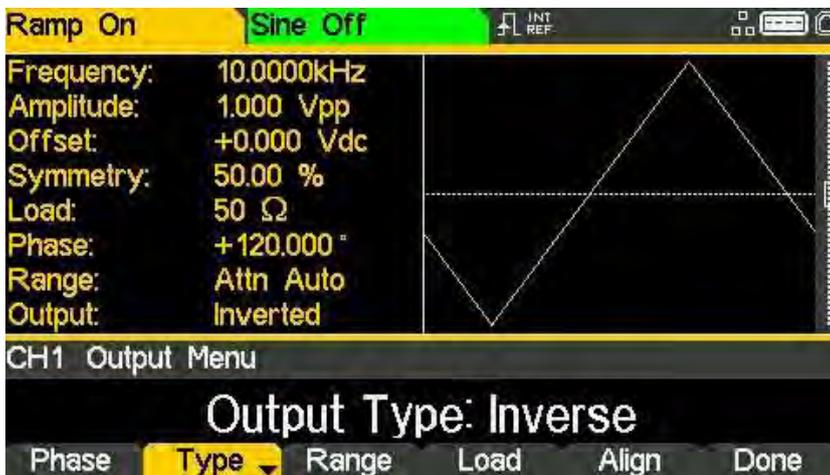
**Inverse** will invert the carrier waveform at the MAIN OUT connector. The output is set to **Inverted** in the parameters box and the carrier waveform in the Graph Box will be inverted.
