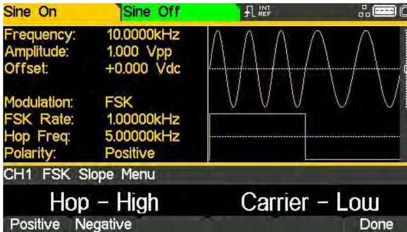
Setting **Negative** will cause FSK to generate the hop frequency while the switching signal is low and the carrier frequency while the switching signal is high.
