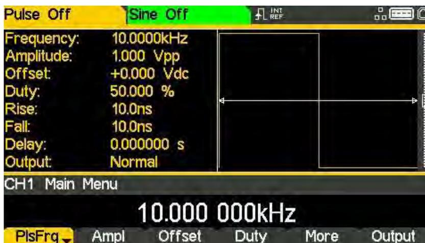
The PlsFrq soft-key allows setting of the pulse frequency. Pressing the key while it is highlighted will change it to PlsPer and the pulse period may be entered. The pulse generator uses its own value for pulse frequency/pulse period. Changing it will not affect the frequency/period value of the other carrier waveforms.
