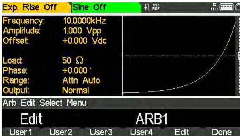
The instrument is capable of performing simple editing of stored arbitrary waveforms. For more complex editing and creation of waveforms see the Waveform Manager Plus V4.13 Windows application, available on the website: [www.aimtti.com](http://www.aimtti.com)
