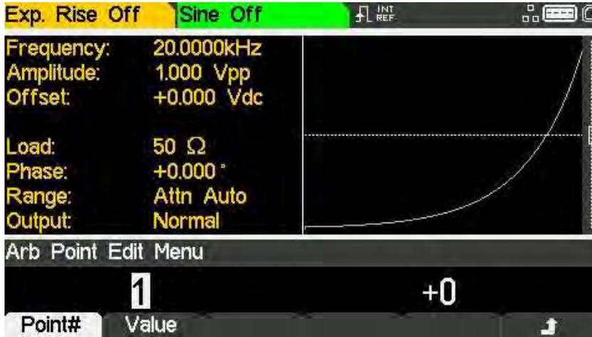
The point edit menu allows individual points in the waveform to be set to any vertical level value. The **Point#** soft-key selects setting of the point number; pressing the **Value** soft-key then enables the value to be changed.
