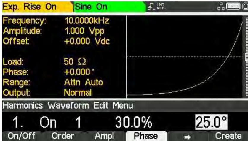
To set the parameters of the next harmonic content press the **→** soft-key. Up to 16 harmonics can be defined, the parameters of which will show with successive presses of the **→** soft-key.
