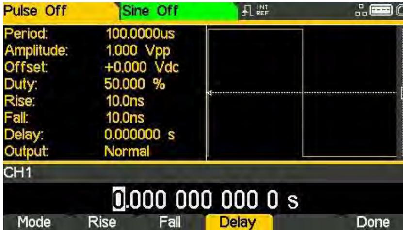
The Graph box shows the delay parameter between the arrows.
