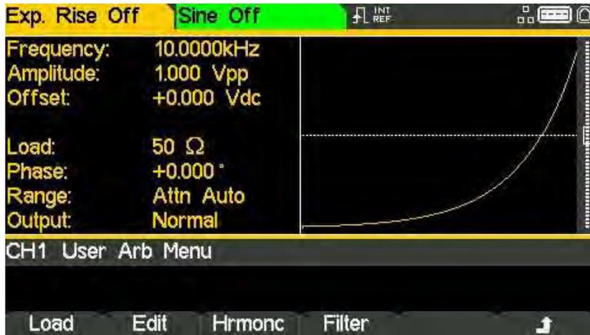
Pressing the Load soft-key opens the load sub-menu.
