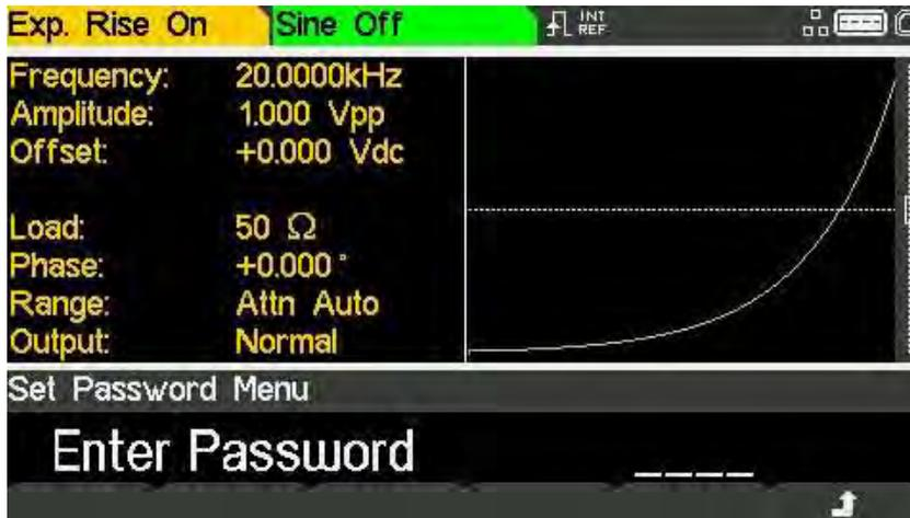
When the correct password has been entered from the keyboard the display changes to the opening screen of the calibration routine and calibration can proceed as described in the Calibration Routine section. If an incorrect password is entered the message **Incorrect Password Please Try Again** will pop up for two seconds before the display reverts to the Utility menu.
