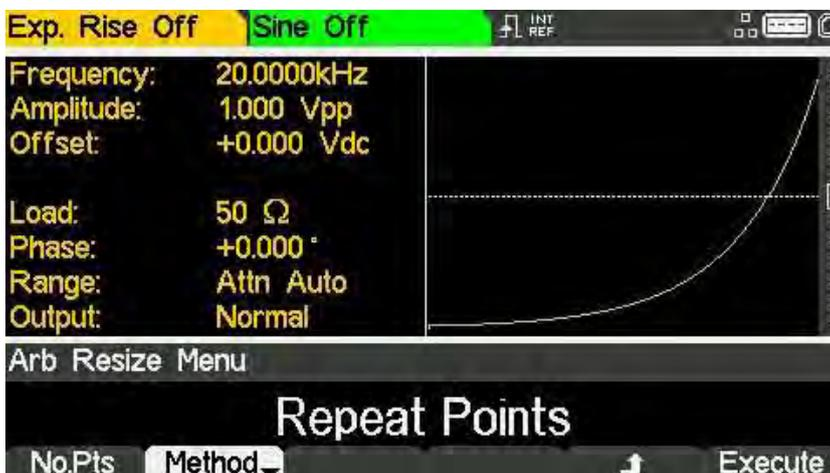
When a waveform is increased in size new points are added between existing points. The way that the values of these new points are calculated depends on the resize method setting. The **Repeat Points** method adds points of the same value as the original point in the waveform. The **Interpolate** method draws a straight line between the existing points.
