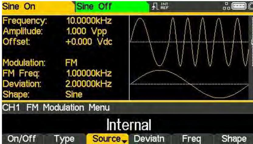
**External** will use the signal present at the MOD IN connector and the **Freq** and **Shape** parameters will no longer be editable. The Graph Box will always show a sinewave as the modulating waveform if the source is set to External.
