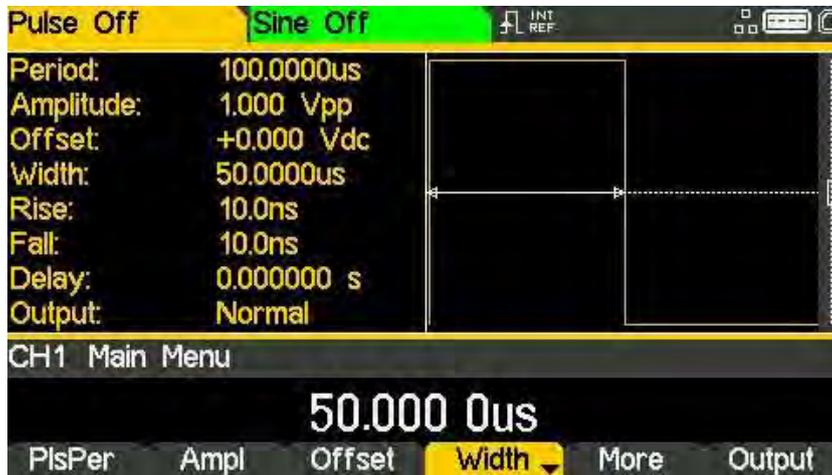
Pressing the **Width** soft-key while it is highlighted changes the editable parameters to **Duty**, the **Duty** parameter is shown in the Edit Box as the width of the pulse as a percentage of the period to a maximum resolution of 0.01%, the Graph Box changes to show that width is being edited and the value is shown in the parameters box.
