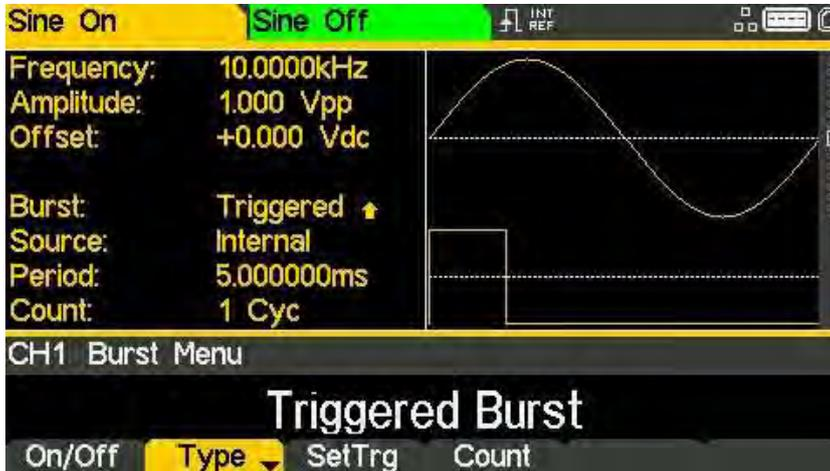
The Parameters Box now shows the current burst parameters of **Burst**, **Source**, **Period**, and **Count**, and **Triggered** is shown in the **Burst** field. The Graph Box shows the burst waveform trigger below a representation of the carrier waveform. The Edit Box contains the selected parameter, in this case **Type**.
