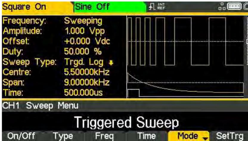
In this mode the sweep will proceed to the end and then waits for a trigger to start again. The soft-keys will change and a trigger waveform will be added to the Graph Box. The Sweep Type field in the Parameters Box will show that the sweep is now triggered.
