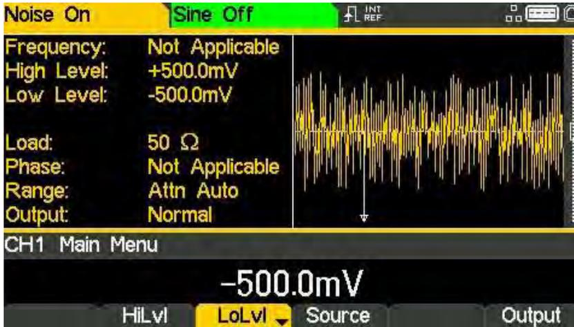
With high/low level mode selected the edit box shows the parameter, the Parameters Box shows High Level and Low Level in place of Amplitude and Offset and the Graph Box changes to show the parameter which is being edited
