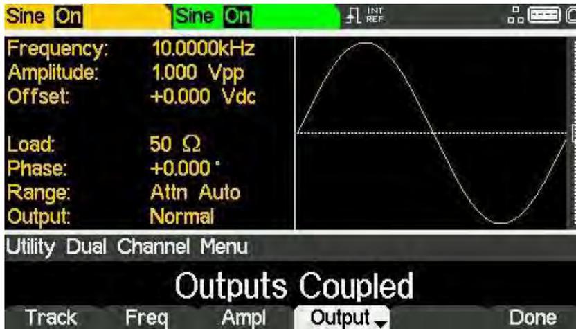
It is possible to set any combination of Frequency, Amplitude and Output coupling.
