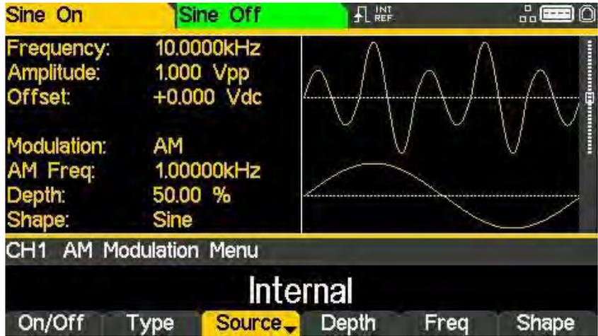
**External** will use the signal present at the MOD IN connector and the **Freq** and **Shape** parameters will no longer be editable. The Graph Box will always show a sinewave as the modulating waveform if the source is set to **External**.
