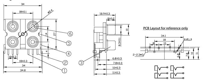
Dimensions : Millimetres Tolerance: ±0.2mm
