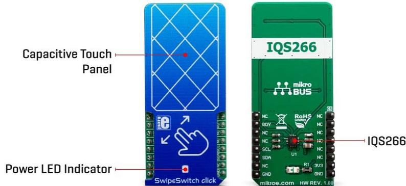
Besides five capacitive touch sensing electrodes, the IQS266 integrates a single proximity channel. This channel can be used to wake up the device from the standby mode when the user approaches the touch panel, ensuring a low overall power consumption that way. CH0 is a dedicated proximity/touch channel and it is treated as a separate channel group in the IQS266 settings. Both proximity and touch thresholds can be defined for this channel.
