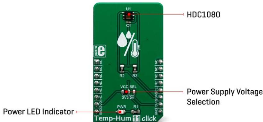
Internally, two sensors are connected to the 14-bit ADC section, which can be set to sample measurements with the resolution of 8, 11 or 14 bits, based on the measurement (integration) time. The OTP memory holds the calibration coefficients that are applied to the measured value and the results are stored on the output registers, in the MSB/LSB format. These values are then used in formulas found in the HDC1080 datasheet so that the final temperature or relative humidity data can be calculated.
