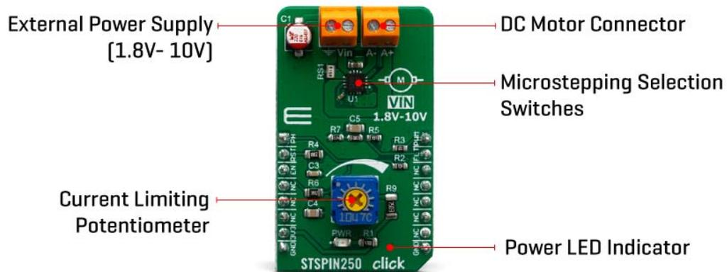
The PWM current controller compares the voltage across the sense resistor ( $V_{SENS}$ ) and the  $V_{REF}$  voltage, which is adjustable on STSPIN250 click. When  $V_{SENS}$  becomes greater than the  $V_{REF}$  voltage, the current limiting is triggered, and the OFF timer starts counting. The decay sequence is performed. By using a simple formula, the  $V_{REF}$  voltage can be determined, for a specific load current:
