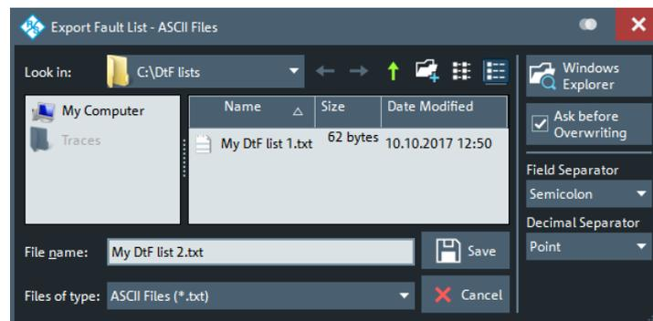
This CSV type file contains one line (terminated by CR+LF) per fault. With ";" as "Field Separator" and "." as "Decimal Separator", the fault list of [Figure 9-4](#) is exported to
