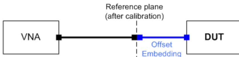
The analyzer can also auto-determine length and loss parameters, assuming that the actual values should minimize the group delay and loss across the sweep range.
