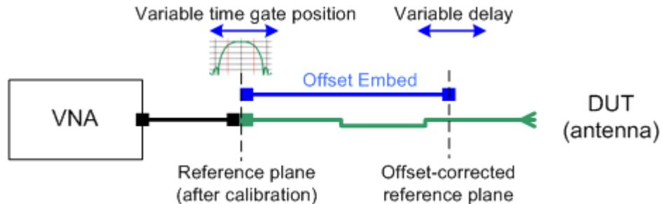
If "Adjust Time Gate" is on, the time gate is moved to left (right) when the offset-corrected reference plane is moved to the right (left). Its absolute position remains fixed. With this setting, it is possible, e.g., to keep the time gate at the position of the antenna connector while the antenna is measured at different length offsets.
