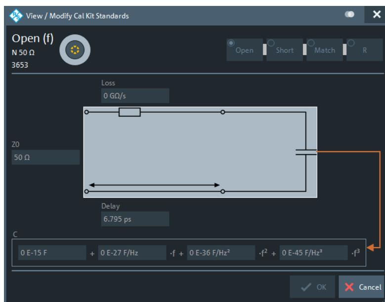
The diagram in the "View / Modify Cal Kit Standards" dialog depends on the standard type for which the dialog was opened. Moreover, it is possible to modify the circuit model using the buttons in the upper right of the dialog.
