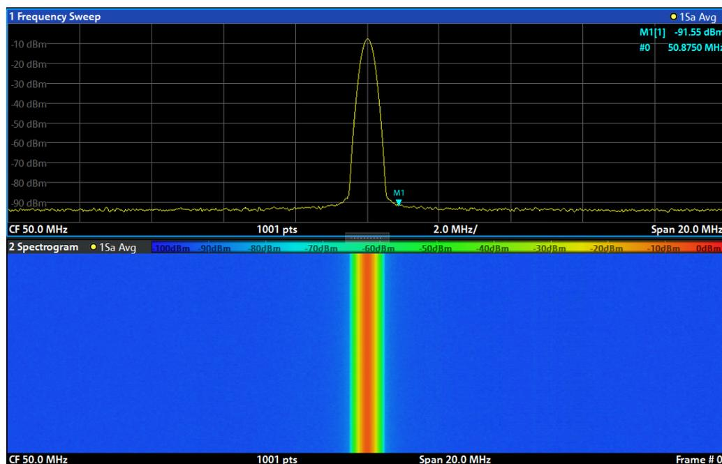
Figure 5-14: Spectrogram of the calibration signal
