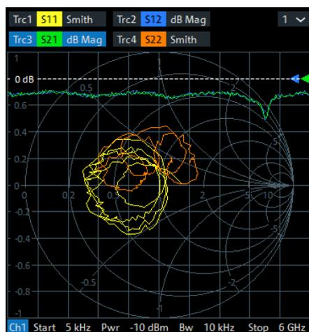
The active trace and active channel is highlighted. The scaling of the axes corresponds to the active trace.
