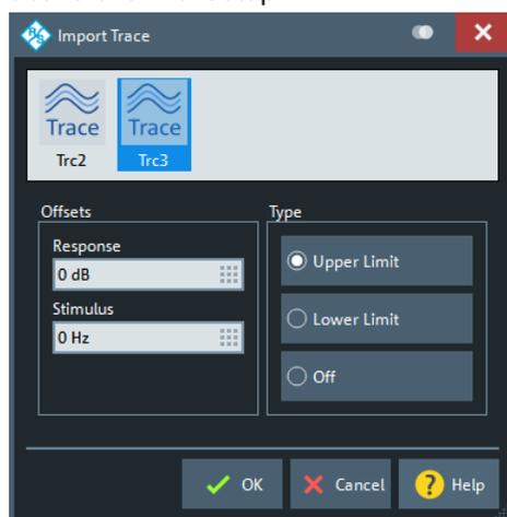
The active trace must be cartesian and the "Format" of the imported trace must be the same as the "Format" of the active trace.
