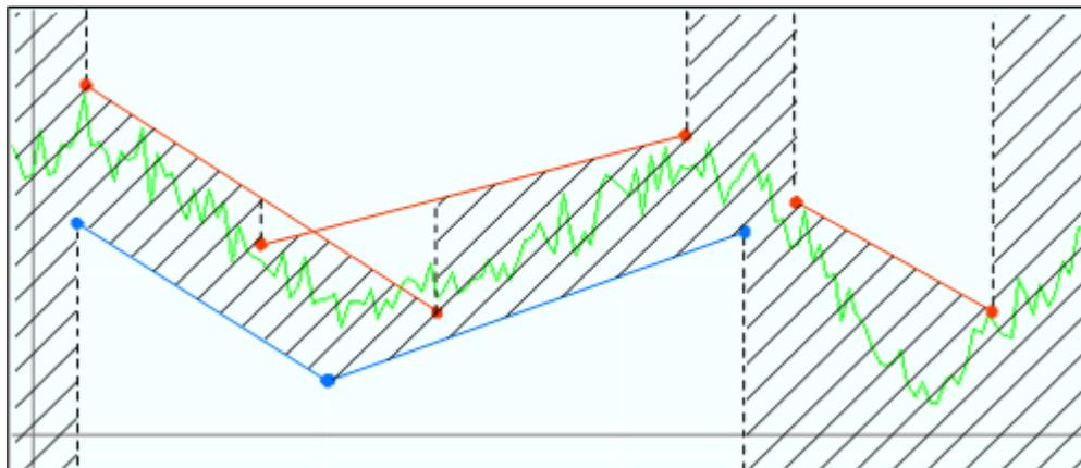
As a consequence of the limit line rules, a DUT always passes the limit check if no limit lines are defined.
