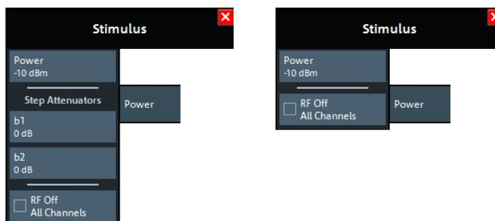
left = R&S ZNL with [Receiver Step Attenuators](#)
