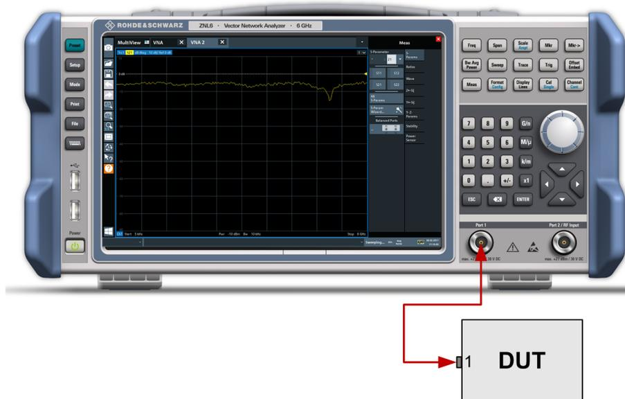
You can also use the basic transmission test setup, e.g. if you want to measure reflection and transmission parameters in parallel.
