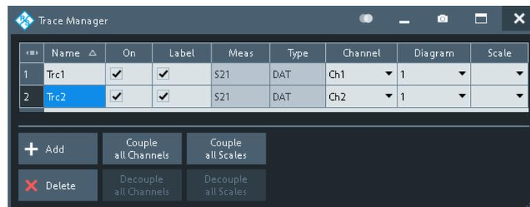
All existing traces of the current channel setup are listed in a table with several editable (white) or non-editable (gray) columns.
