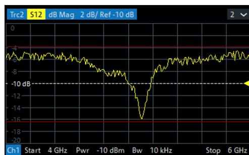
**Note:** Display of the limit line and limit check are independent of each other: Hiding the limit line does not switch off the limit check.
