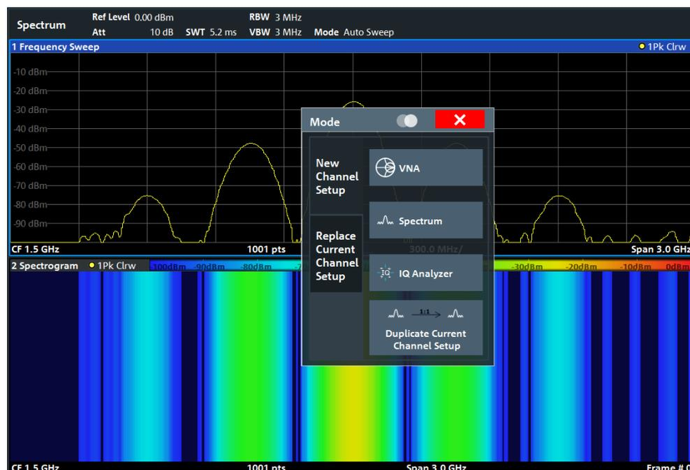
Figure 5-8: Adding a new channel setup
