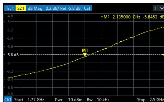
2. Open the [Mkr->] > "Peak" softtool tab and activate "Min" search. The marker jumps to the absolute minimum of the curve in the entire sweep range. The marker info field shows the coordinates of the new marker position.
