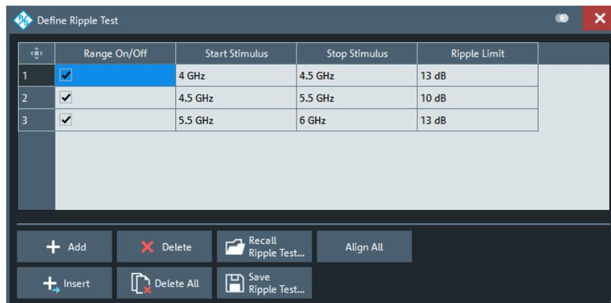
The "Define Ripple Test" dialog contains a table to edit the individual ranges of the ripple check ranges. The buttons below the table extend, shorten, or reorder the range list and save/recall ripple test data.
