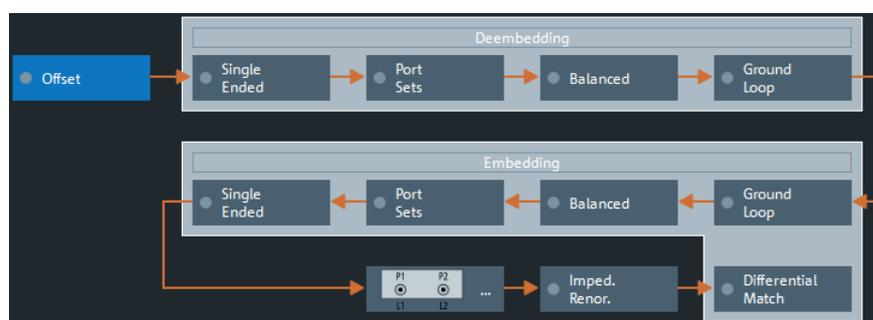
Figure 8-4: De-/Embedding calculation flow
