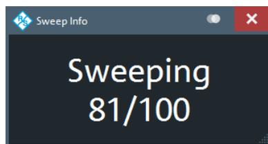
The possible sweep stages and how they are displayed partly depend on the selected sweep mode (see "[Continuous / Single](#)" on page 320):
