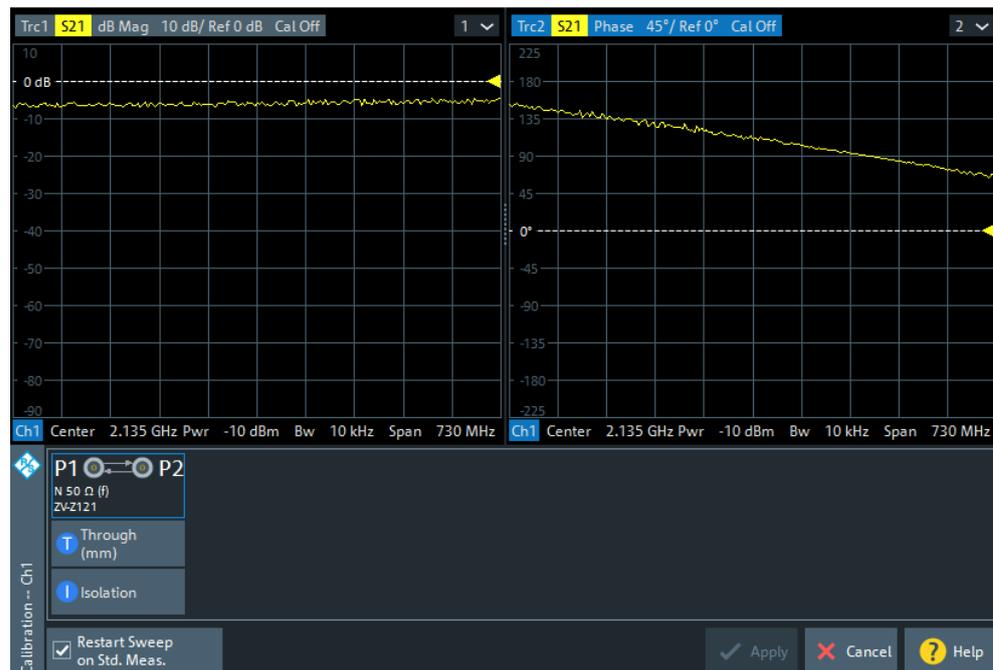
The analyzer performs a calibration sweep for the measured quantity  $S_{21}$ . The magnitude and phase of the result is displayed in two diagrams, together with the expected typical result for a Through standard. The similarity of real and expected traces indicates that the Through standard has been properly connected. After the R&S ZNL/ZNLE has completed the calibration sweep and calculated the correction data, the "Apply" button is enabled.
