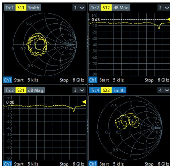
If less than two (three / four) traces are available, the new diagrams are created with a default trace. Dual (triple / quad) split corresponds to "Split Type: Tile Horizontal" with 2 (3 / 4) diagrams.
