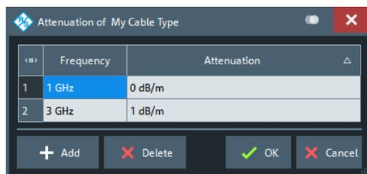
Given the specified attenuation values the R&S ZNL/ZNLE calculates the attenuation factor at the center of the channel's sweep range and corrects the impulse response trace using this attenuation factor *Attenuation* ( $f_{center}$ ).
