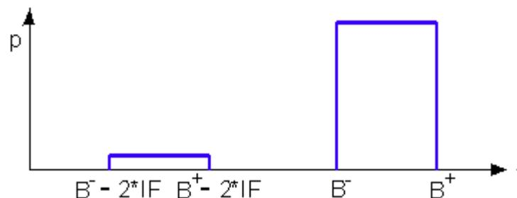
For a wide bandpass, the spurious response flattens the filter edges.
