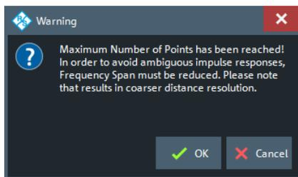
"OK" reduces the frequency span  $\Delta f$  to
