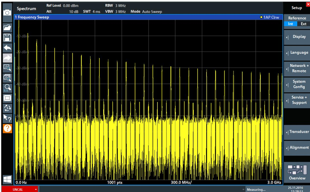
Figure 5-12: Calibration signal with optimized display settings
