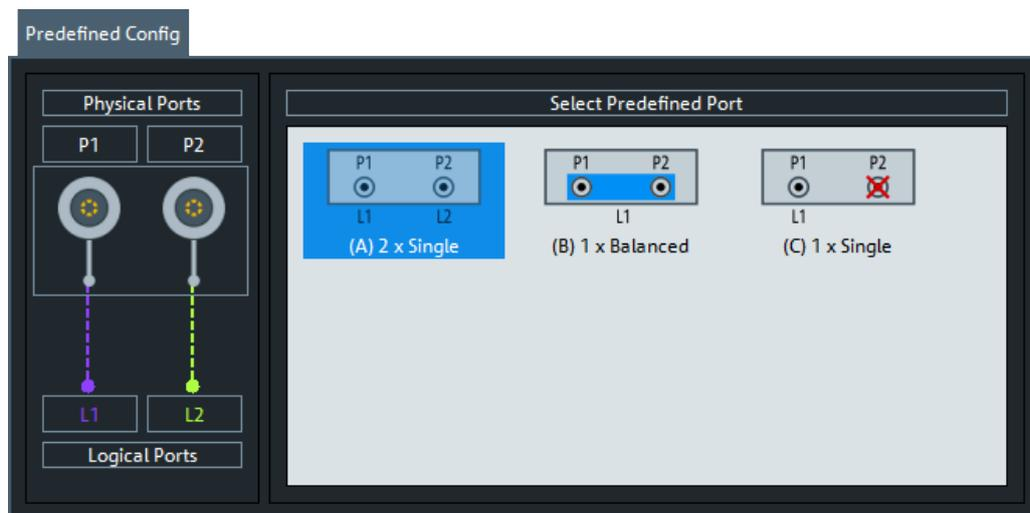
The port configurations are arranged in the list to the right. The resulting port assignment is shown on the left-hand side of the "Predefined Config" tab.
