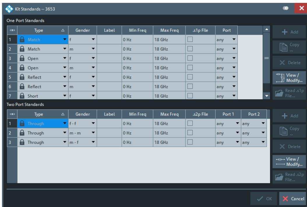
One port and two port standards are listed in two separate tables. Most of the buttons on the right side are available only if the "Kit Standards" dialog was opened for a user-defined calibration kit.
