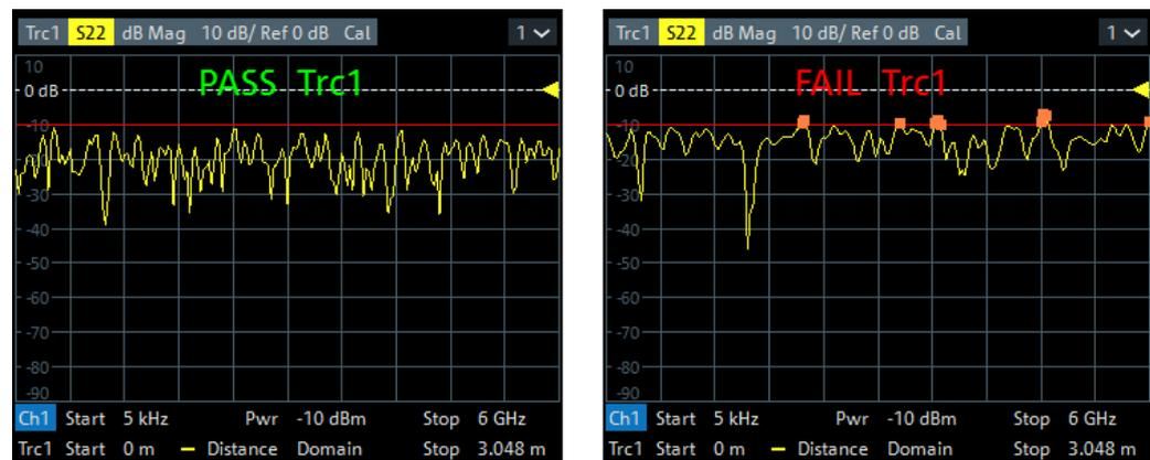
**Note** that the fault limit is handled like any other limit line. When "Fault Limit Check" is enabled, the current "Fault Limit" forms a new upper line segment replacing other previously defined limit lines (see [Chapter 9.9.4.2, "Define Limit Lines Dialog"](#), on page 402).
