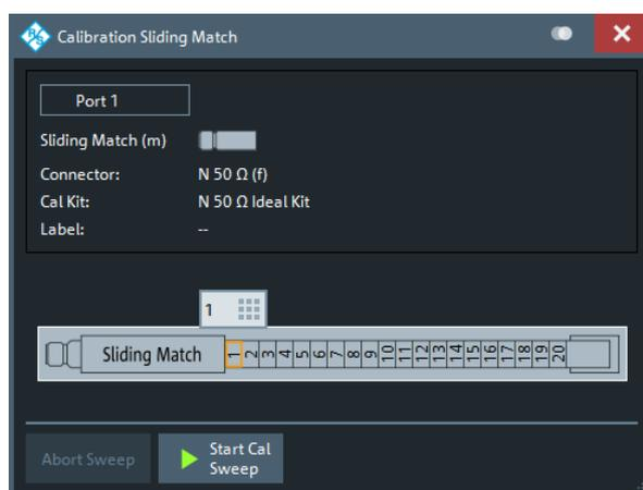
Figure 8-2: Sliding Match: GUI representation
