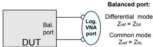
The "Balanced Ports" dialog allows you to switch to balanced operation and to define the reference impedances the differential and common mode.
