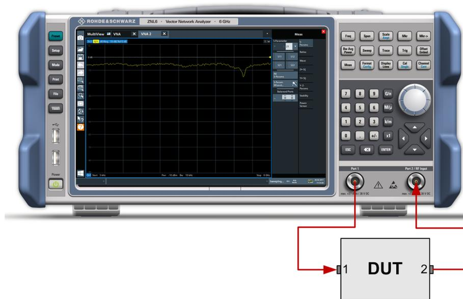
1. Connect the DUT between test ports 1 and 2 of the network analyzer as shown above.
