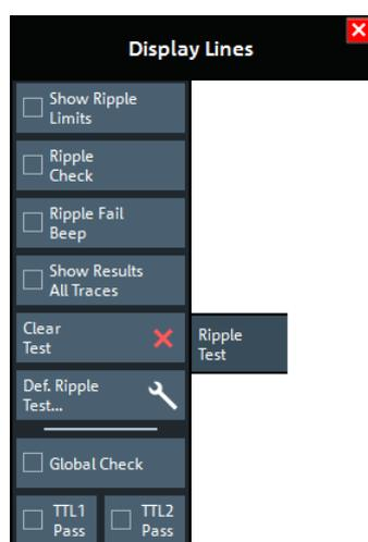
The "Def. Ripple Test..." button opens the "Define Ripple Test" dialog (see [Chapter 9.9.5.2, "Define Ripple Test Dialog"](#), on page 408).
