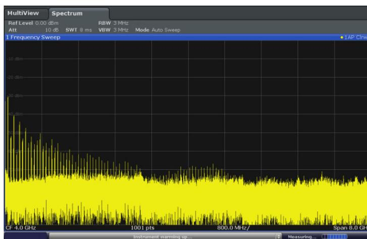
Figure 5-11: Calibration signal as RF input
