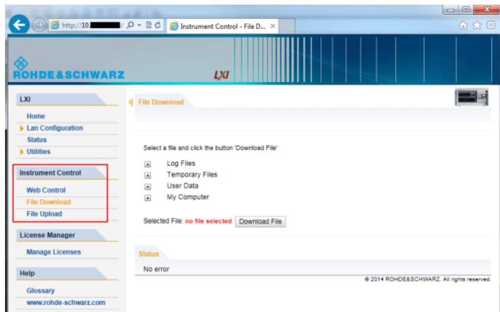
The most commonly used folders on the instrument are displayed, for example those that contain user data, as well as the top-most *My Computer* folder, from which you can access all other folders on the instrument.
