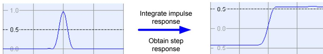
The step response is recommended for impedance measurements and for the analysis of discontinuities (especially inductive and capacitive discontinuities). The impulse response has an unambiguous magnitude and is therefore recommended for most other applications.
