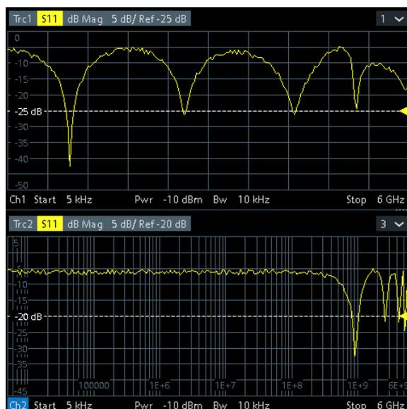
Figure 8-1: S11 trace in dB Mag format: sweep type Lin Freq (top) and Log Freq (bottom)
