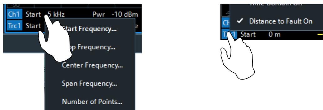
E.g. "Distance to Fault" can also be enabled/disabled via the context menu of the trace label (touch and hold for more than one second).
