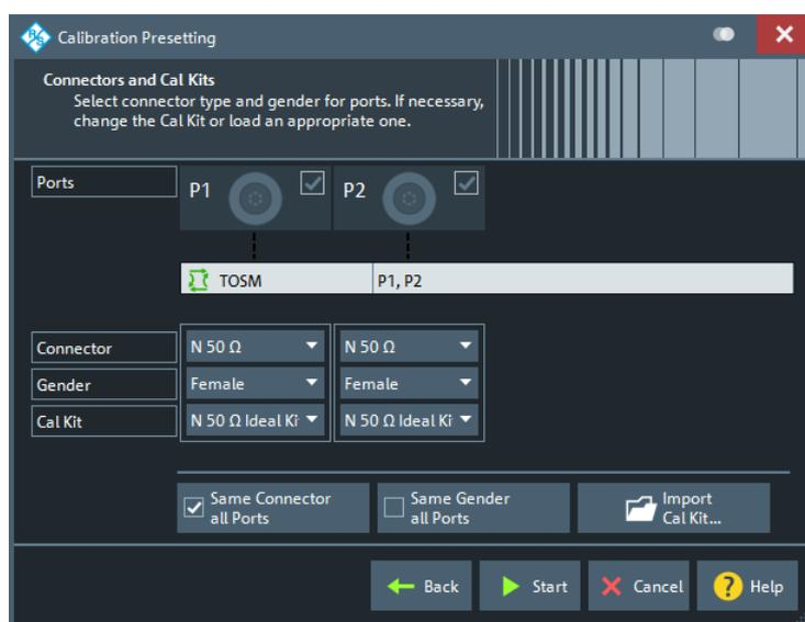
Figure 9-13: Calibration Setting Wizard, Step 2: Connectors and Cal Kits
