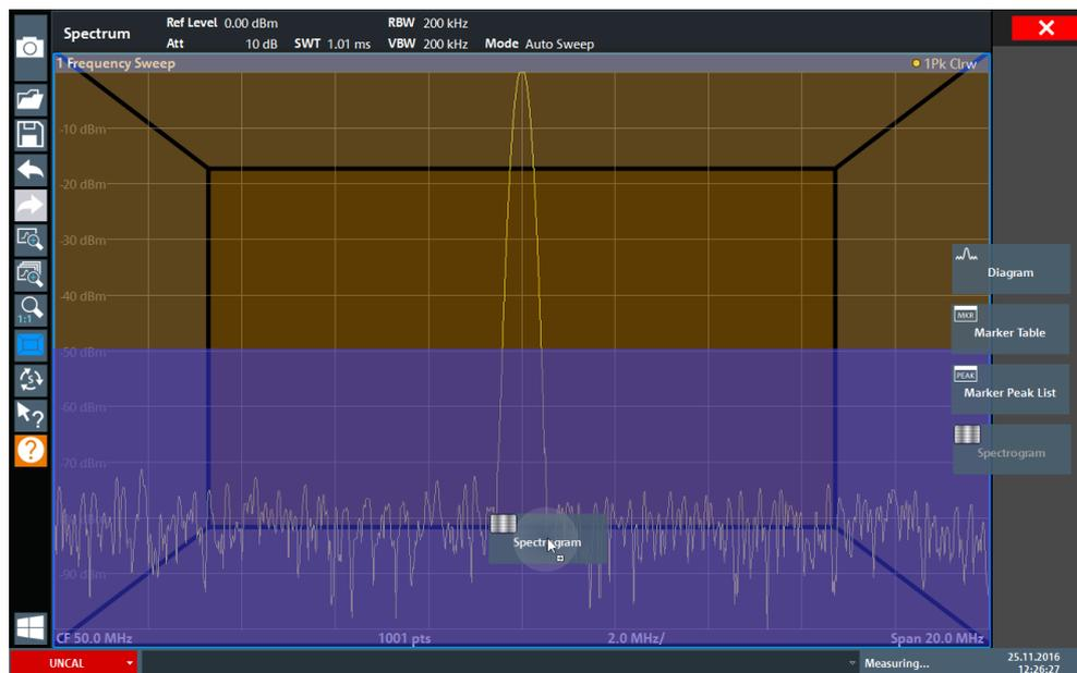
Figure 5-13: Adding a Spectrogram to the display
