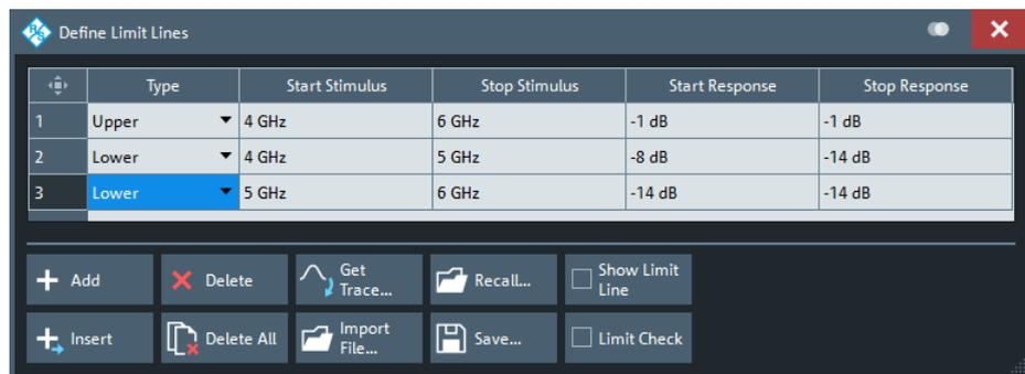
The "Define Limit Lines" dialog contains a table to edit the individual segments of the limit lines. The buttons below the table extend or shorten the segment list.
