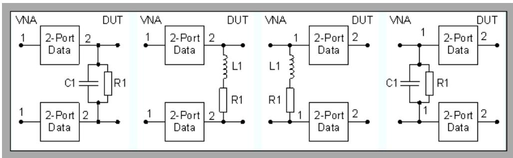
The following networks are composed of two serial Cs or Ls (as seen from the analyzer test port), followed by a shunt C or L. They are named Serial Cs, Shunt C / Serial Cs, Shunt L / Serial Ls, Shunt C / Serial Ls, Shunt L.
