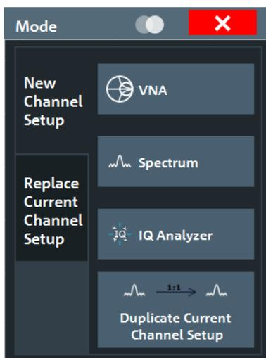
Figure 6-1: Defining Channel Setups (R&S ZNL with R&S ZNL-B1)
