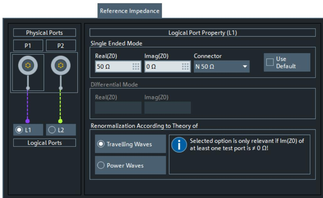
By default, the reference impedance of a physical port is set to the reference impedance of the connector type assigned to the port. However, it can be defined as an arbitrary complex value (renormalization of port impedances). By changing the reference impedance, it is possible to convert the measured values at 50 Ω (75 Ω) into values at arbitrary port impedances.
