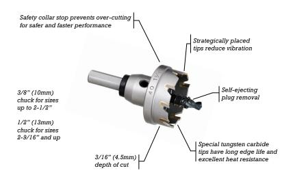
Tungsten carbide tips have excellent wear and heat resistance. Light, smooth cutting entry with great boring speed.
