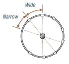
Variable tip placement reduces vibration.
