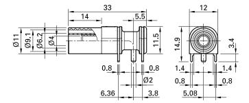
For mounting on printed circuit boards, touch-protected according to IEC/EN 61010-1. The socket is directly soldered onto printed circuit boards. The right-angled configuration minimizes the force transmitted to the printed circuit board through theplugged-in test lead. Right-angled Ø 4 mm rigid socket accepting spring-loaded Ø 4 mm plugs with rigid insulating sleeve.
