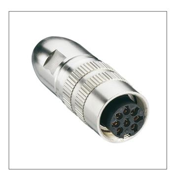
Socket acc. to AISG specification and IEC 61076-2-106, IP68, with threaded joint and solder terminals, shielded at 360°
