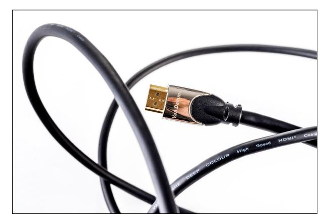
The Van Damme HDMI cable range comprises High Speed, High Speed with Ethernet and active Redmere High Speed with Ethernet assemblies. All are HDMI 2.0 compatible for use with display resolutions up to 4K 60 Hz 4:2:2. The flexible precision cable has individually screened foam skin polyethylene insulated TMDS pairs with additional overall foil and dense copper braided screen, ensuring accurate transmission.
