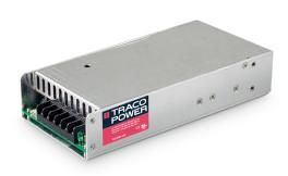
The TXH 600 series models are very compact 600 Watt universal power supplies. Rear side IEC-C13 line socket including mains switch and fuse and the output screw terminal make the connection of these power supplies very easy. Sense line, auxiliary output, remote control, adjustable output voltage, and load share line for up to 3 units in parallel make the units all-purpose applicable.
