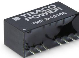
The TMR-2E series is a family of isolated 2 W dc-dc converter modules with regulated output, featuring wide 2:1 input voltage ranges. The product comes in a compact SIP-8 plastic package with small footprint occupying only 2.0 cm<sup>2</sup> (0.3 square in.) of board space.
