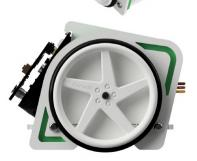
**STEP 3:** Push the Servo:Lite board fully back inside the :MOVE mini.
