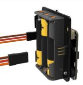
**STEP 1:** Plug the servo cables back into the Servo:Lite board. The left servo should plug into the left-hand side of the board and vice versa. The cables should be threaded down the gaps on either side as shown below.
