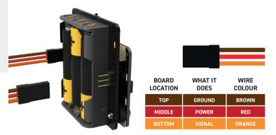
**STEP 2:** With both wheel servos plugged in, it is time to write some test code. Set out the servos like below. This will allow trimming/calibration of the servos. This means they will stop and travel at the same speed when commanded.
