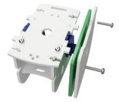
**STEP 5:** Turn the assembly upside down, align the smaller rectangular holes of the side panels up with the protruding bars on the base plate, and slot them together. Drop M3 nuts into the T-joints, and secure with the 16mm bolts.
