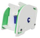
**STEP 7:** Add a wheel (built earlier) and screw the smallest servo screw through the middle to secure it to the servo.
