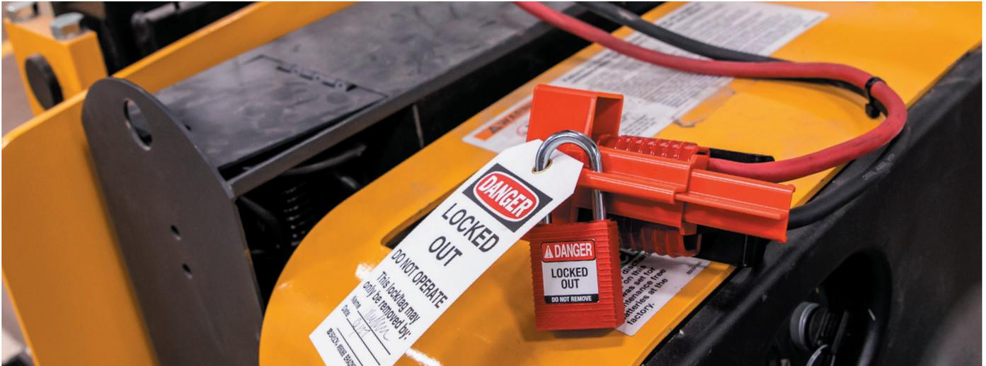
For forklift safety, proper operation is certainly a main concern, but a secure lockout during maintenance can be just as important. With the BatteryBlock Power Connector Lockout, you ensure both by keeping your forklift locked out and locked down. **Unlike current products on the market, this device fits on 175A and 350A power connectors with and without handles.**
