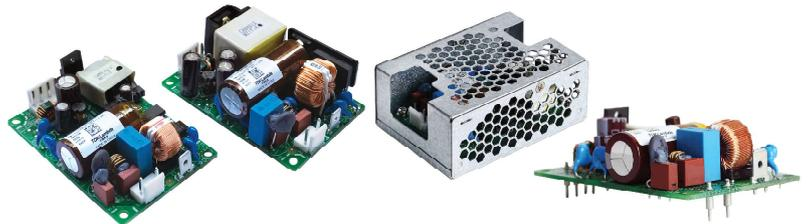
The CUS30M and CUS60M are 2" x 3" footprint AC/DC power supplies with outputs ranging from 5V to 48V. They are certified to IEC60601-1 3rd edition (medical), IEC60950-1 and IEC60335-1 with compliance to EN60601-1-2:2015 Edition 4 immunity requirements. Rated at 30W and 60W, these compact products meet class B conducted and radiated EMI in either a Class I or Class II (double insulated) construction, without the need for external filtering.
