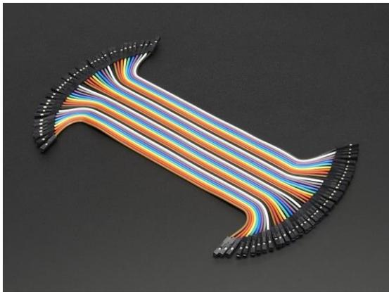
Handy for making wire harnesses or jumpering between headers on PCB's. These premium jumper wires come in a 'strip' of 40 (4 pieces of each of ten colors). They have 0.1" contacts on either end and fit cleanly next to each other on standard-pitch 0.1" (2.54mm) header. We recently updated these so they are in a 'ribbon strip' instead of individual wires. You can always pull the ribbon wires off to make individual jumpers, or keep them together to make neatly organized wire harnesses.
