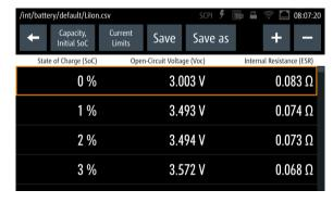
2. Go back to the main menu and select "Channel 1". Scroll down to "Battery Simulator", switch it on and open the settings. Select "Load from file..." and load the settings of the Lilon battery as described before. Switch back to the channel display and expand it to display channel 1 only.
