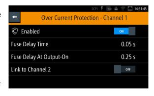
The sensitivity of the fuse is specified using the "Fuse delay time". This allows users to modify the behavior of the power supply to prevent a channel from being switched off due to a short current spike during operation."
