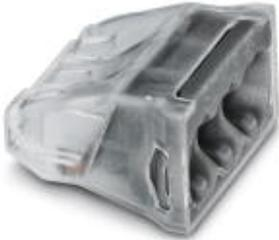
3-pos. socket terminal block with spring-cage connection, for toolless wiring with push-in connection method, for one and multi-strand conductors with a cross section of 0.5 to 2.5 mm<sup>2</sup>, insulation housing transparent.
