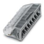
8-pos. socket terminal block with spring-cage connection, for toolless wiring with push-in connection method, for one and multi-strand conductors with a cross section of 0.5 to 2.5 mm², insulation housing transparent.
