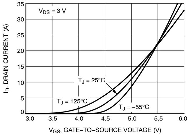
Figure 2. Transfer Characteristics
