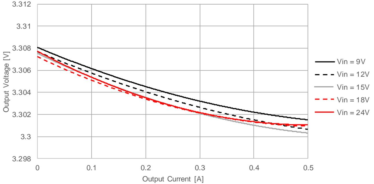
173950336 Load Regulation  $V_{OUT} = 3.3V$ ,  $T_A = 85^\circ C$
