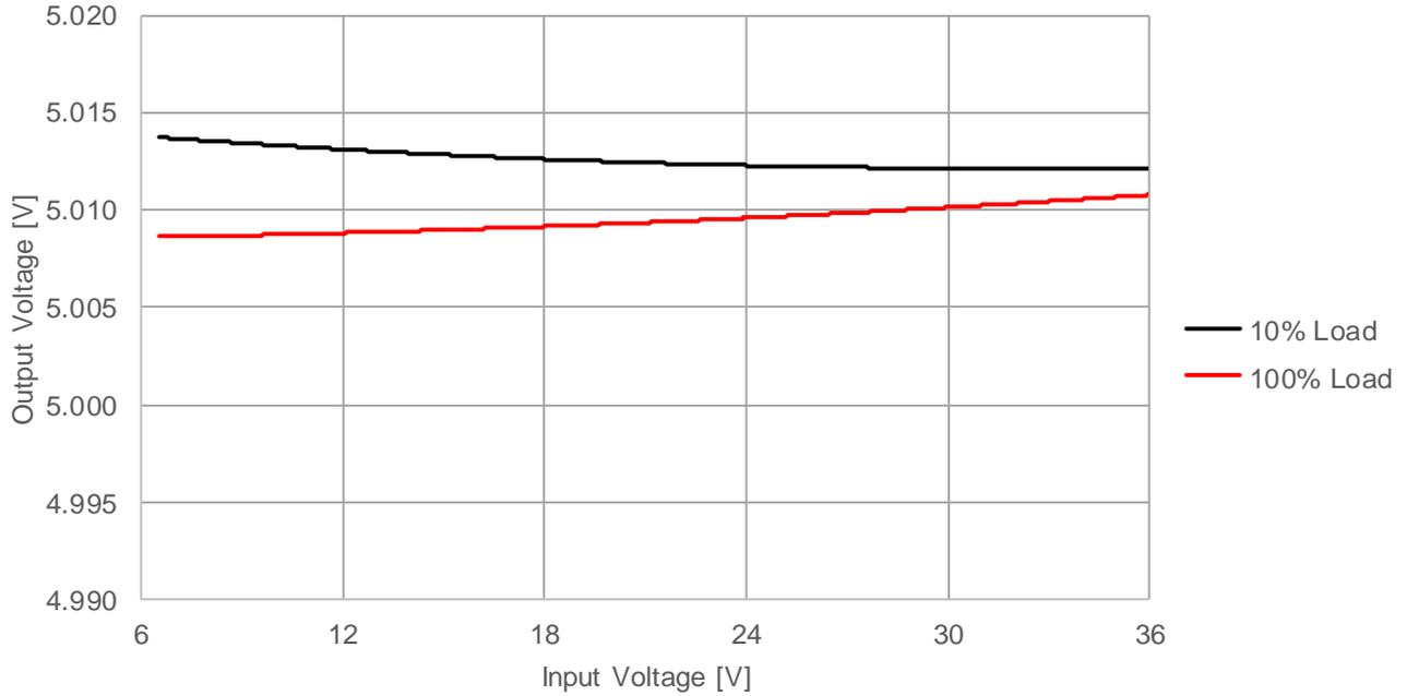
173950536 Line Regulation  $V_{OUT} = 5V$ ,  $T_A = 85^{\circ}C$
