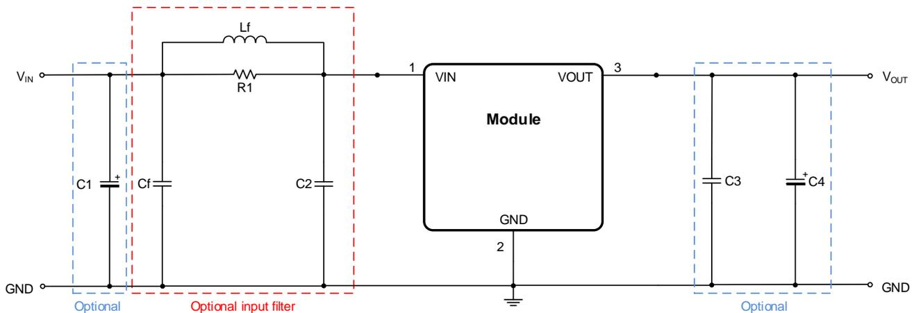
The 17950x36 partially integrates both the input and output capacitors. It is also recommended to use a 10 $\mu$ F input capacitor C2 for high impedance input wires or traces and 22 $\mu$ F output capacitor C3 for applications where a low output voltage ripple is required.
