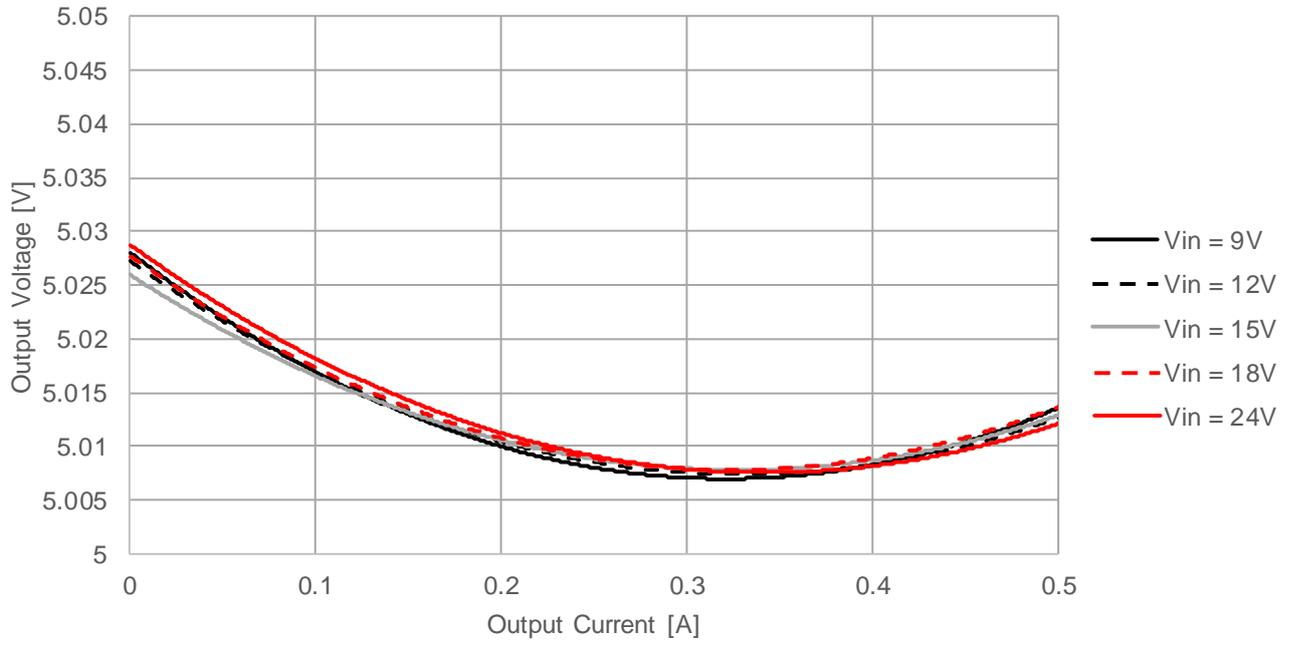
173950536 Load Regulation  $V_{OUT}=5V, T_A = 85^\circ C$
