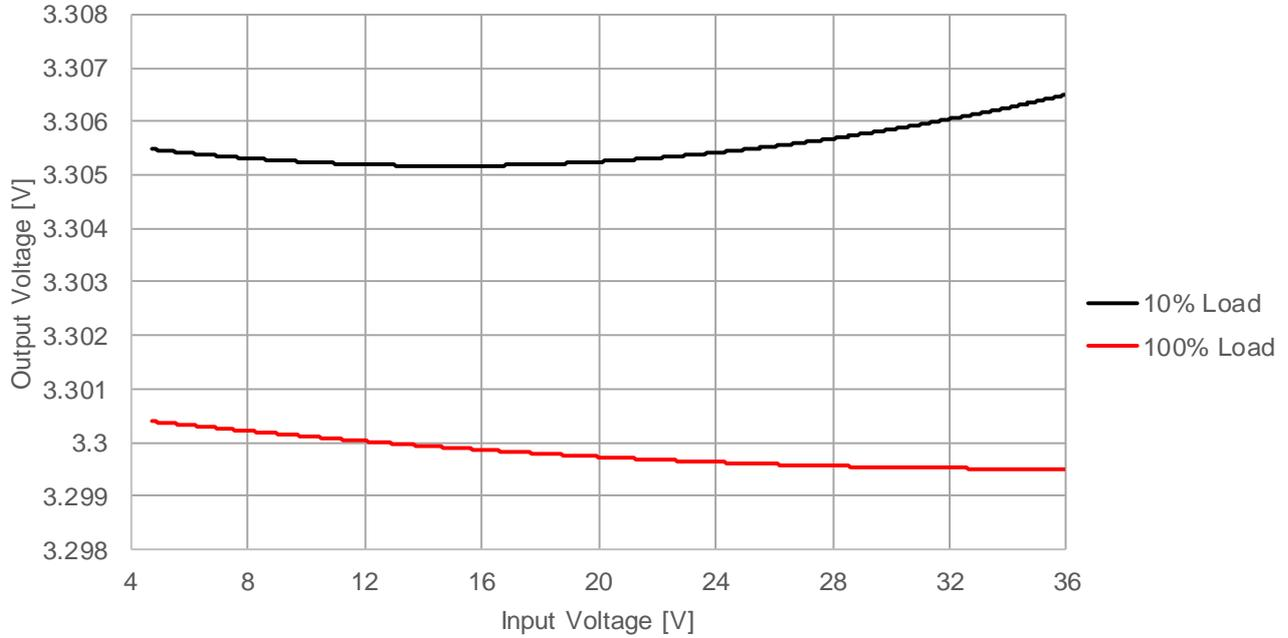
173950336 Line Regulation  $V_{OUT} = 3.3V$ ,  $T_A = 85^\circ C$
