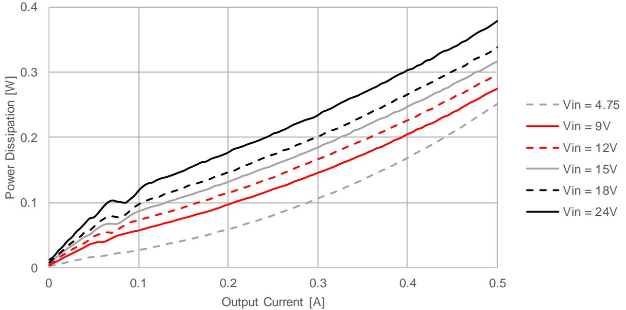
173950336  $V_{OUT} = 3.3V$ ,  $f_{SW} = 710kHz$ ,  $T_A = 85^{\circ}C$
