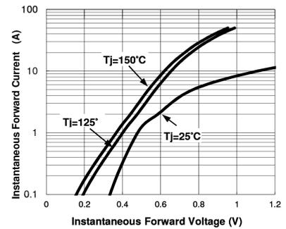
Figure 3. Typical Instantaneous Forward Characteristics Per Leg
