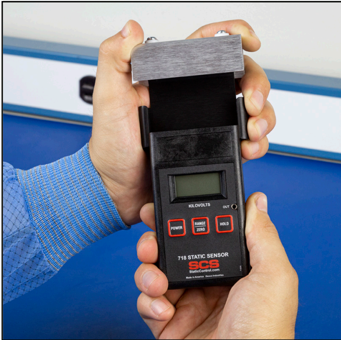
Figure 3. Sliding the Conductive Plate onto the Static Sensor
