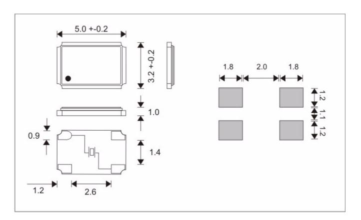
Holder Style Mode Adjustment Tolerance Temperature Stability Operating Temp. Range Load Capacitance ESR Static Capacitance (C0) Ageing Marking 5x32x1 4-Pad Fundamental ± 30PPM at 25°C ± 30 PPM -20°C to +70°C 18 pF 100 Max Ohm Unspecified pF +/-5ppm 1st Year Max AEL8.057 ww/yy
