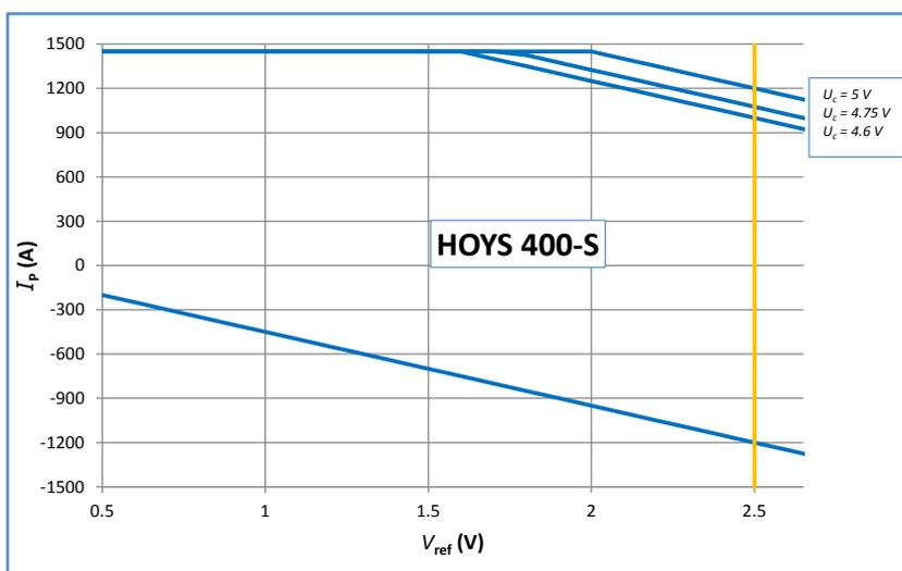
Measuring range versus external reference voltage
