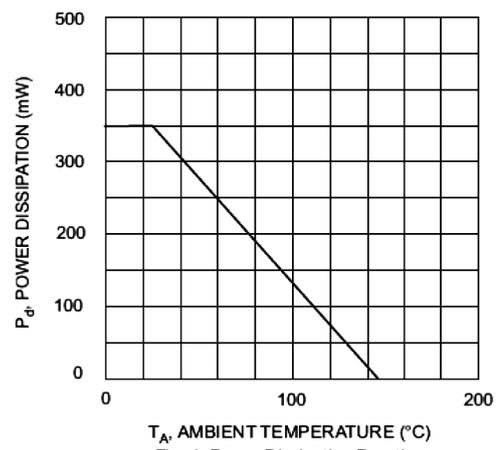
Fig. 4 Power Dissipation Derating
