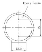
Dimensions : Millimetres Tolerance: ±0.5mm
