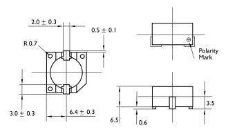
Dimensions : Millimetres Tolerance: ±0.5mm
