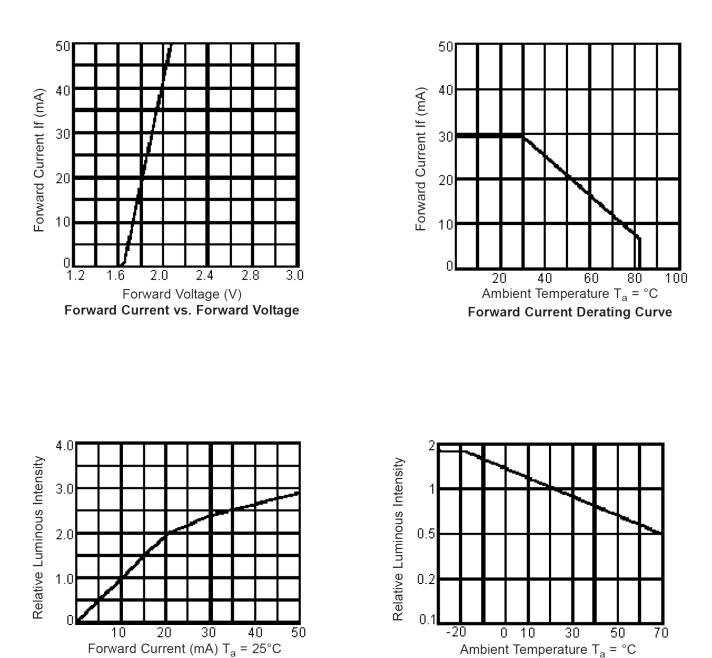
Luminous Intensity vs. Forward Current
