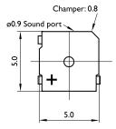
Dimensions : Millimetres Tolerance: ±0.5mm
