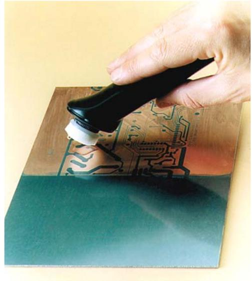
Three applicators each containing safe, ready-to-use PCB chemistry, which offers a clean and efficient alternative to processing in trays. Each applicator is sealed with a valve mechanism terminated by a sponge which dispenses precisely the right amount on the board. All applicators work at room temperature, are waste free, and when exhausted can be disposed of without any special precautions.
