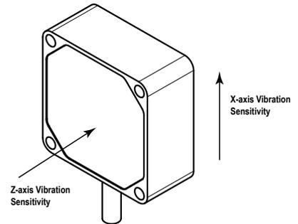
After determining the sensor direction and location, mount the sensor for the best possible vibration sensing accuracy.
