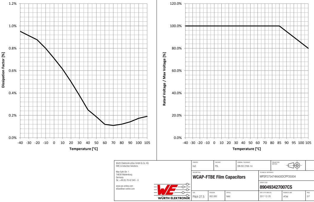
**Rated Voltage vs. Temperature:**
