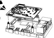
Lower the upper casing over the assembly until it snaps into place.
