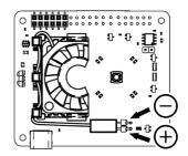
Clip the PCB onto the mounting pillars ensuring the riser pins locate through the holes in the board.
