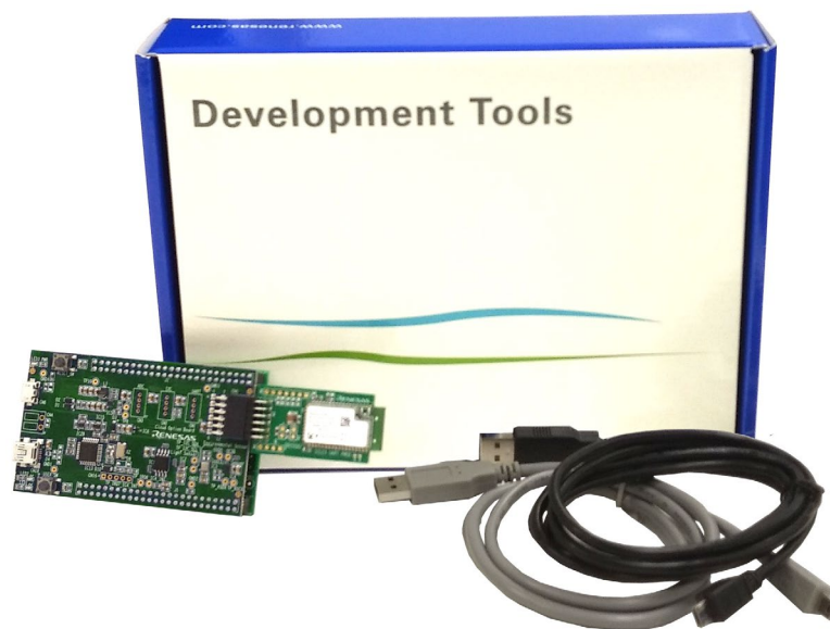
Figure 3: The Renesas RX65N starter kit with cloud option board and Pmod Wi-Fi module (source Renesas Electronics Corp.)
