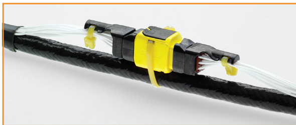
369 Connectors Can Be Easily Secured with Cable Ties, Eliminating the Need for Additional Hardware or Cutouts
